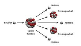
1. **Absorbing a Neutron**: For fission to happen, the unstable nucleus, like uranium or plutonium, first absorbs a neutron. Think of the neutron as a tiny particle that, when added to the nucleus, makes it so unstable that it splits.
