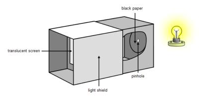
The pinhole camera is a very simple piece of apparatus that demonstrates several points about the physics of light. The pinhole camera was first used in about 1000 AD and since then it has been a simple way of producing a correct image of a scene. Artists from the sixteenth century onwards used a pinhole camera to help them get the correct proportions for a painting.
