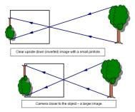
A bigger pinhole will allow more light to get in and so the image will become brighter, but it will also be blurred. This is because light from one point on the object can reach more than one point on the screen.
